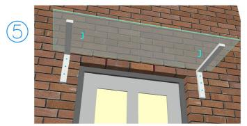
J Remove pre-assembled fixings from the brackets. Sit glass onto the brackets.
